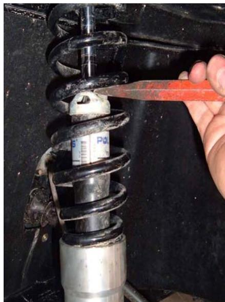
This shows how to push the strut down on the PVC spacer. You may have to apply pressure to the strut on some installations. When you have the strut seated on the spacer tighten the lower pinch bolt.
