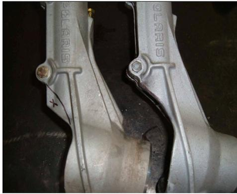
On the left is a stock knuckle marked for removal and on the right is one with the material removed. Removing this material will not affect the integrity of the knuckle. And is not necessary on later models.
