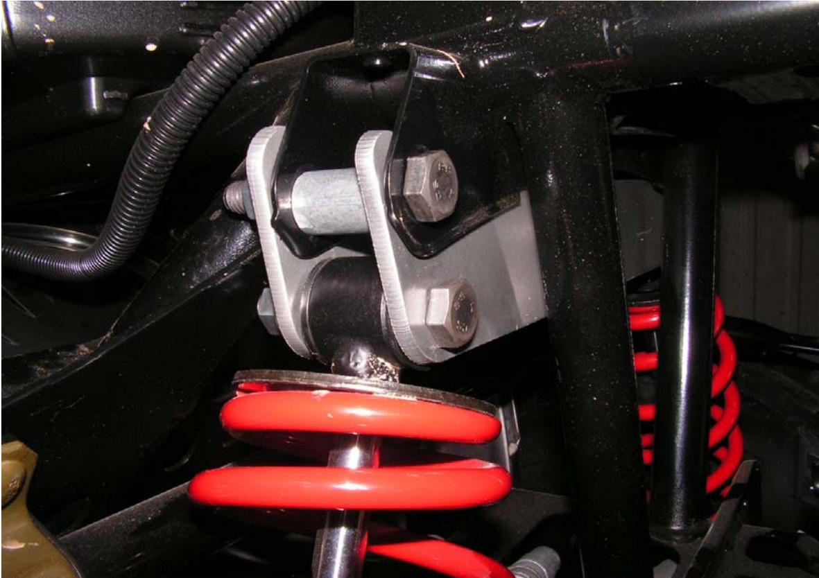
7.) Install tire/wheel and lower back onto floor. Install the new sway bar links using the supplied hardware. You will re use the factory bushings and washers.
