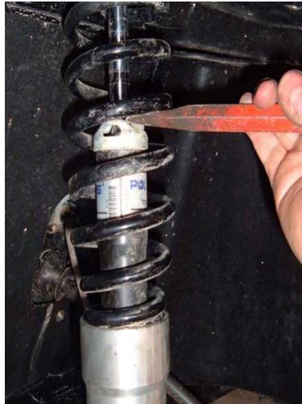
**This shows how to push the strut down on the PVC spacer. You may have to apply pressure to the strut on some installations. When you have the strut seated on the spacer tighten the lower pinch bolt. REAR Disassembly / Reassembly**
