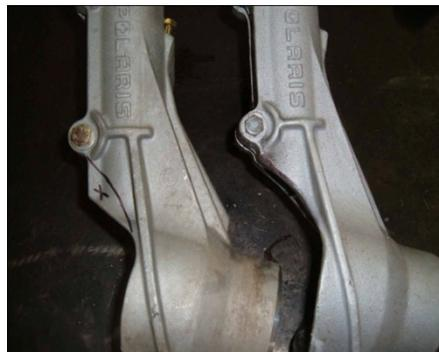
On the left is a stock knuckle marked for removal and on the right is one with the material removed. Removing this material will not affect the integrity of the knuckle.
