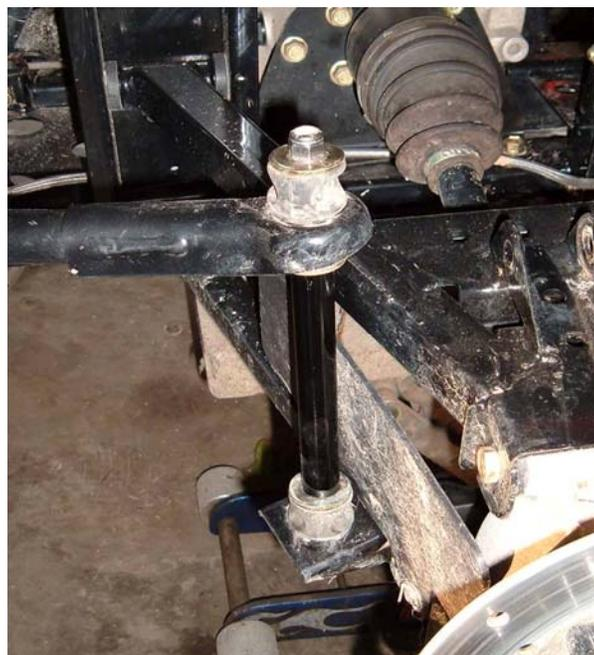
19.) Reconnect the sway bar one side at a time insert the new bolt through the bushings as they came off use the new tube furnished in place of the stock aluminum link. Do not tighten when you do one side wait until you have the bolts and sleeves installed on both sides before you tighten. Tighten the nut on the bolt until you get swelling of the bushings.
