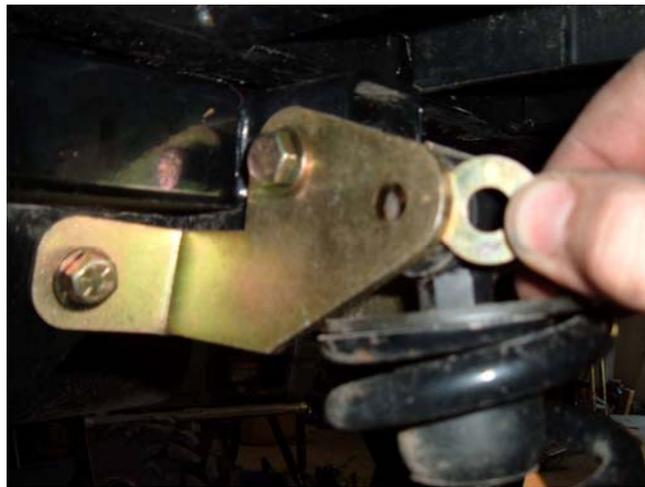
18.) Reinstall the shocks and be sure to install the washer included as shown one on each side of the shock.
