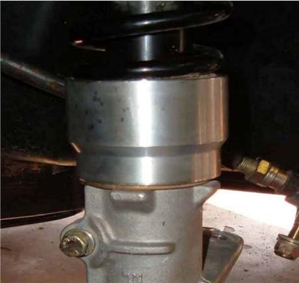
The PVC spacer is inserted into the aluminum strut housing. The strut is inserted and fully seated down against the PVC spacer. The Urethane spacer is installed onto the strut housing, with the factory steel washer underneath it. The spring is sitting inside the lip of the Urethane spacer
