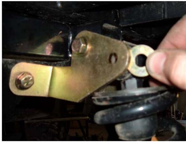
7) Reinstall the shocks and be sure to install the washer included as shown one on each side of the shock
