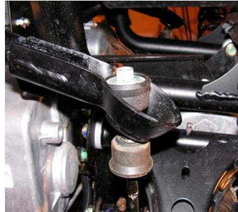
***NOTE:*** We recommend if the primary use of your RZR is for mud ridding, rock climbing or slow trail riding, that you completely remove both the front and the rear sway bar. Removing the sway bar will allow the machine to perform better in these situations.
