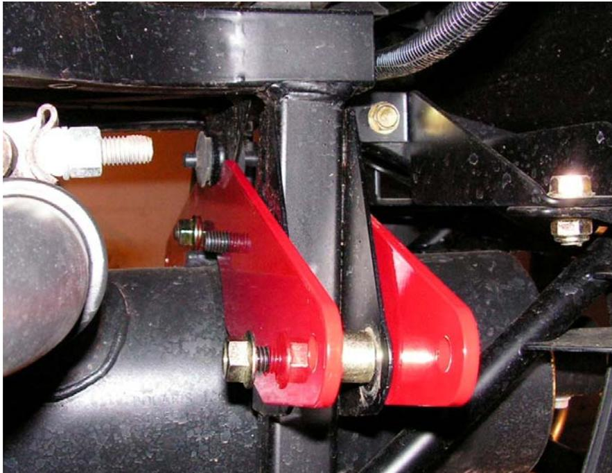
9.) Refer to **Diagram #5 & #6** Disconnect the swaybar links from the swaybar. Remove the sway bar completely and flip over before reinstalling. Do not flip the attaching bracket, just the sway bar. *Pay attention to the muffler locating tabs going through the bracket, make sure they are reinstalled correctly.* After reattaching at the frame, reinstall the sway bar links.
