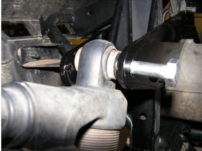
10.) **Refer to Diagram #4 & #5** Disconnect the sway-bar links from the sway-bar. Remove the sway bar completely and flip over before reinstalling. Do not flip the attaching bracket, just the sway bar. *Pay attention to the muffler locating tabs going through the bracket; make sure they are reinstalled correctly.* After reattaching at the frame, reinstall the sway bar links.
