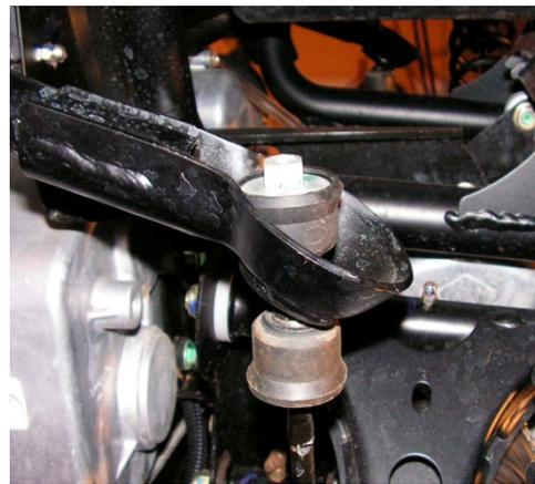
**NOTE:** *We recommend if the primary use of your RZR is for mud riding, rock climbing or slow trail riding, that you completely remove both the front and the rear sway bar. Removing the sway bar will allow the machine to perform better in these situations.*
