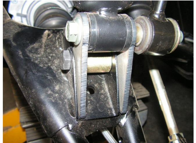
**In Diagram #1, the notch is on the left side of the bracket, driver's side is shown.**
