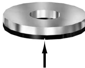
**Rubber must face plastic when installing Sealing Washers**
