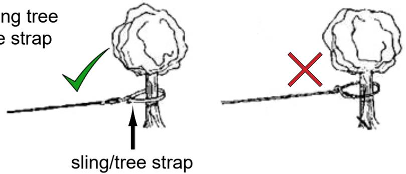
Do not winch from an acute angle. Synthetic Rope will pile up on one side of Winch Drum causing damage to Synthetic Rope and Winch.
