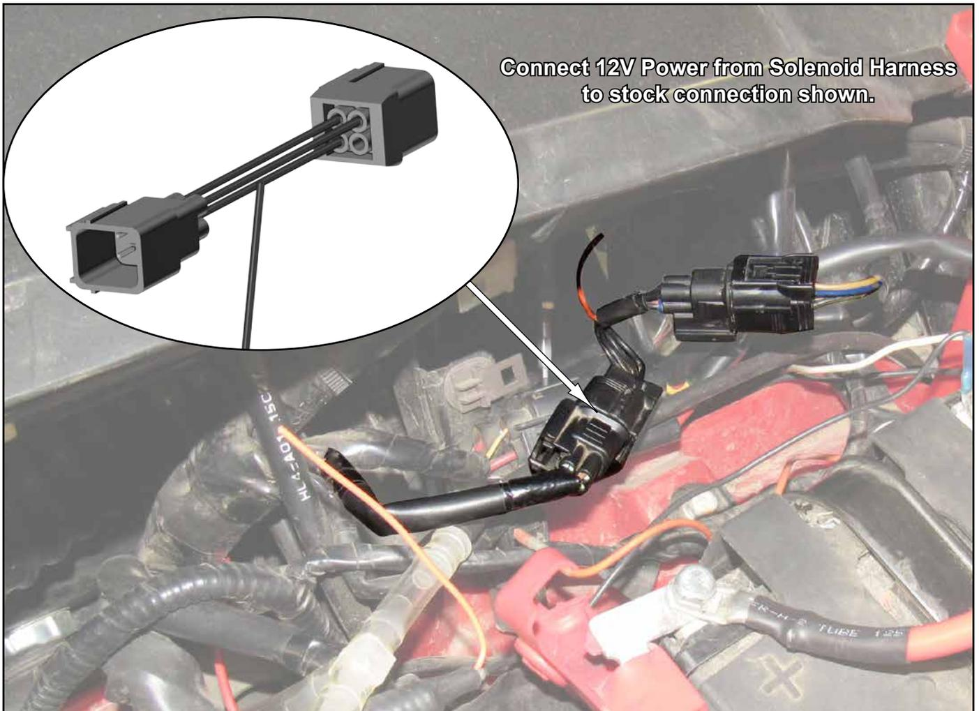
Connect 12V Power from Solenoid Harness to stock connection shown.
