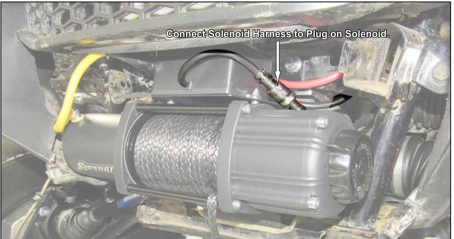
Connect Solenoid Harness to Plug on Solenoid.
