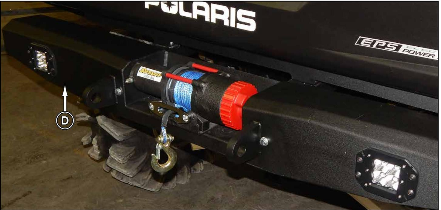
**Install Winch to Bumper (D) with components and hardware supplied with Winch.**
