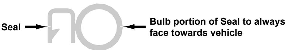
Soak Seal in hot water before cutting or installing to increase flexibility.
