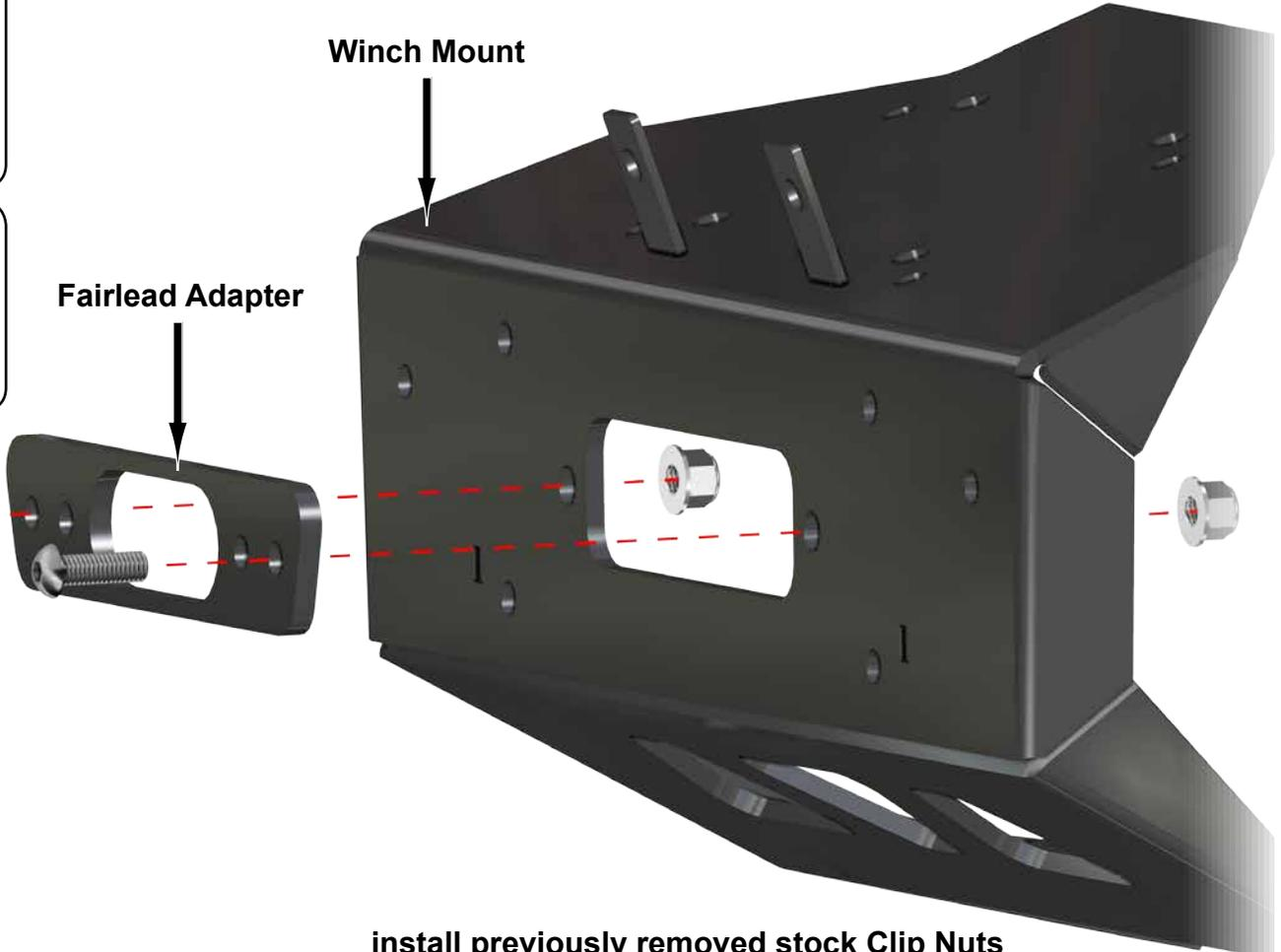
install previously removed stock Clip Nuts
